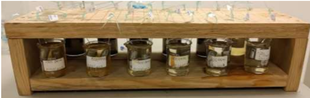
Figure 1.2 1018 steel specimens subjected to weight loss analysis
